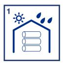
Store Croptight in original protective sleeve. Store reels on their sides in a dry place out of direct sunlight. The ideal storage temperature is 20 – 30OC. Keep reels in sleeves and condition at ambient temperature prior to use
