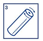
Reels should only be removed from protective packaging immediately prior to use. Open sleeve using the tear strip provided. The arrow on the reel end indicates the direction of wrapping.
