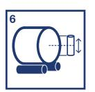
The balewrap being applied over Croptight must have at least a 50% overlap. Check carefully that each layer overlaps at least half the previous layer. 750mm films should overlap by at least 31cm.
