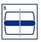
The Croptight reel must be placed centrally in the Intake unit so that the centre of the reel aligns with the middle of the bale.
