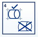
The baled material must always be evenly distributed over the width of the baler pick up. Bales should be dense and cylindrical in shape. The more compact the bale, the better the forage preservation will be.
